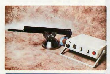
The single-barreled prototype, shown here with firing mount and casing in place, has a basic payload of 15 9mm projectiles. The electronic firing console, at right, controls the weapon's all-out rate of fire of up to 45,000 rounds per minute.
